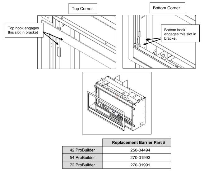
• Remove the glass frame following the directions below.
