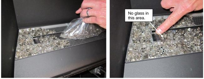
Make sure the rear and end air channels are free of crushed glass. Use a screwdriver to clear this area. <u>Make sure the glass is only 1 layer deep on the burner.</u>
