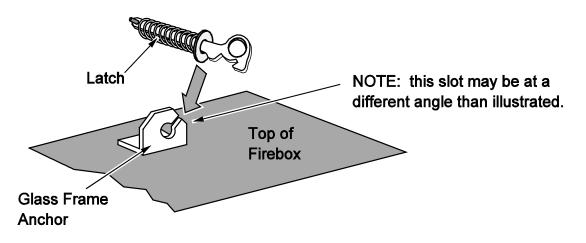
Note how the washer on the latch fits behind the flange on the glass frame anchor.
