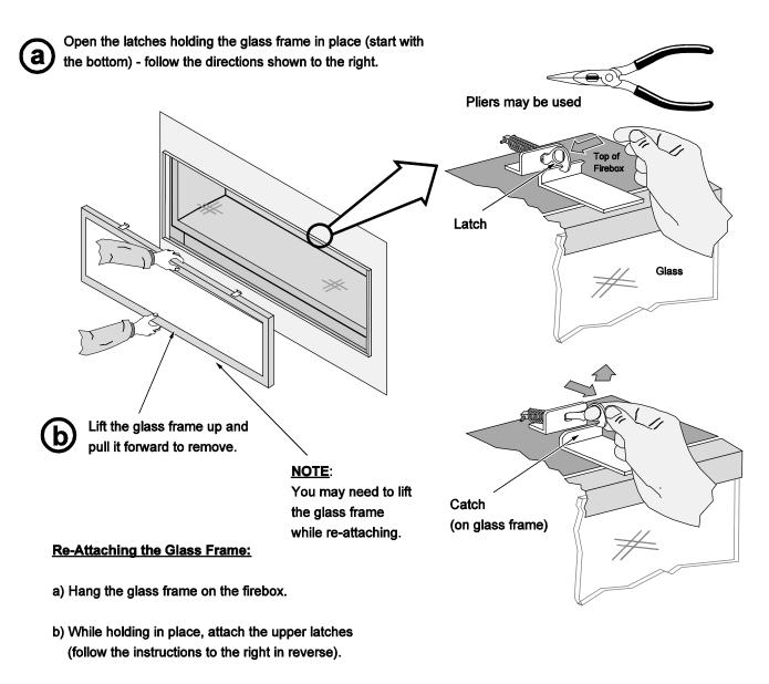
c) Lift the glass frame slightly and attach the lower latches.
