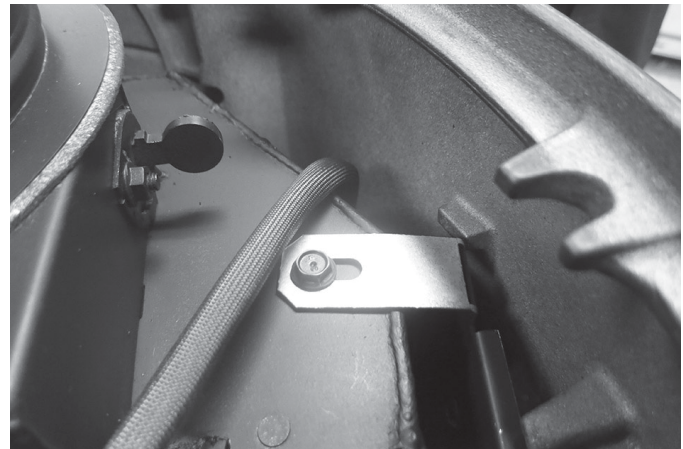
Figure 16.2. Remove the firebox-to-side plate bolt.
