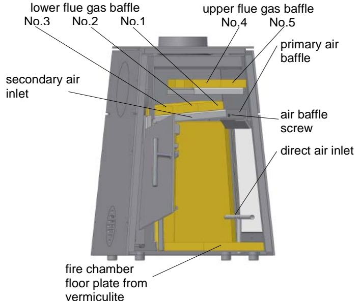
*Replacing the vermiculite plates:*
