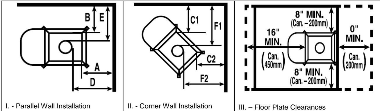
\*Note that the Parallel Wall and Corner Wall Installation clearances (diagrams I. and II.) are based on the dimensions at the top of the stove - 16" (40cm) wide x 14" (35cm) deep.
