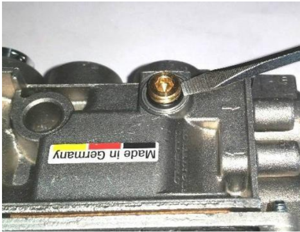
Figure 22 – Low Flow Orifice Removal – O-ring
