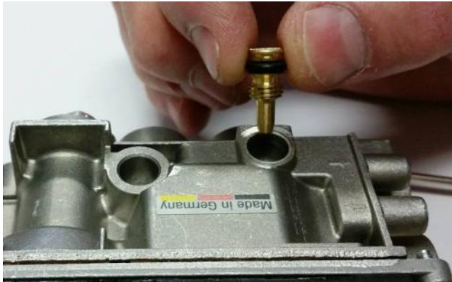
Figure 23 – NG Low Flow Screw Removal
