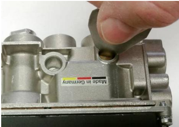
Figure 25 – Tighten LP Low Flow Orifice
