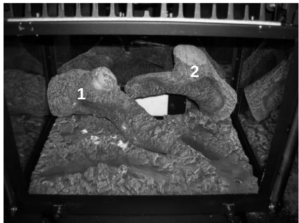
Figure 32 – Log 2 in Position
