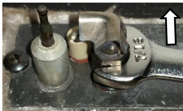
Figure 26 – Pilot in NG (Pilot Gate forward)
