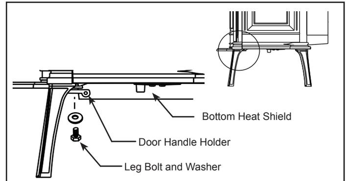
**Figure 21** - Handle holder and heat shield positions.
