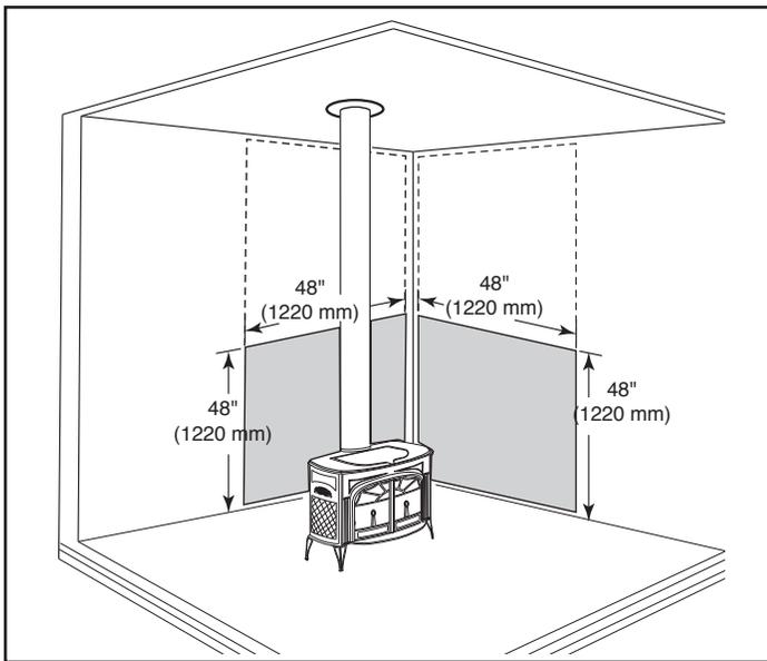
**Figure 16** - Parallel installation, vertical chimney connector, two wall shields. Reduced clearances for both rear and side walls. Wall shields may meet at corner if desired. Shielding for connector is centered behind connector.
