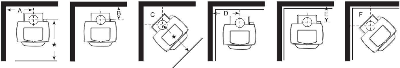
\* This distance, from the center of the flue collar to the front edge of the hearth, is the same for all installations on this page: 34" (865 mm) in the United States and 36" (914 mm) in Canada.
