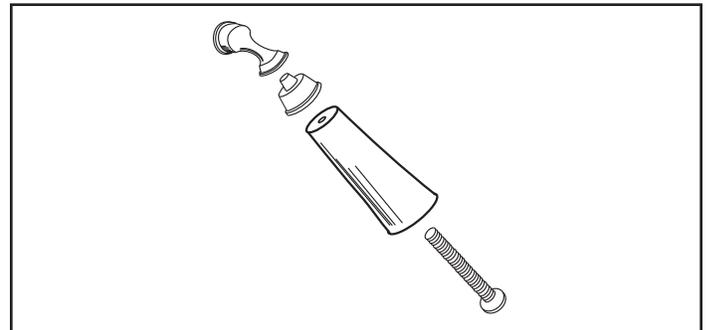
Figure 26 - Assemble the front door handle.
