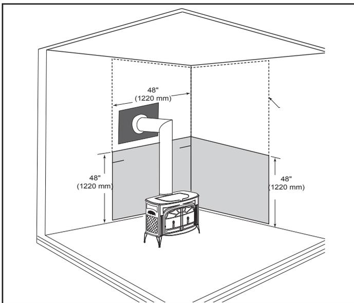
**Figure 17** - Parallel installation with rear wall pass-through, two wall shields. Reduced clearances to both rear and side walls. Wall shields may meet at corner if desired. Wall pass-through must comply with codes.
