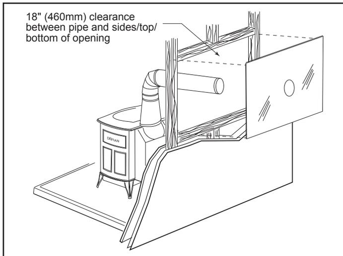
**Figure 11** - An approved wall pass-through for Canada.
