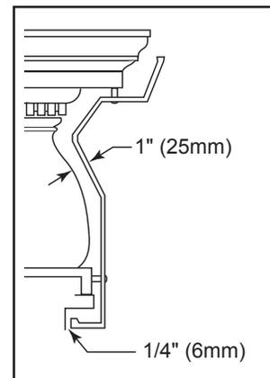
Figure 14 - A custom-formed mantel shield.
