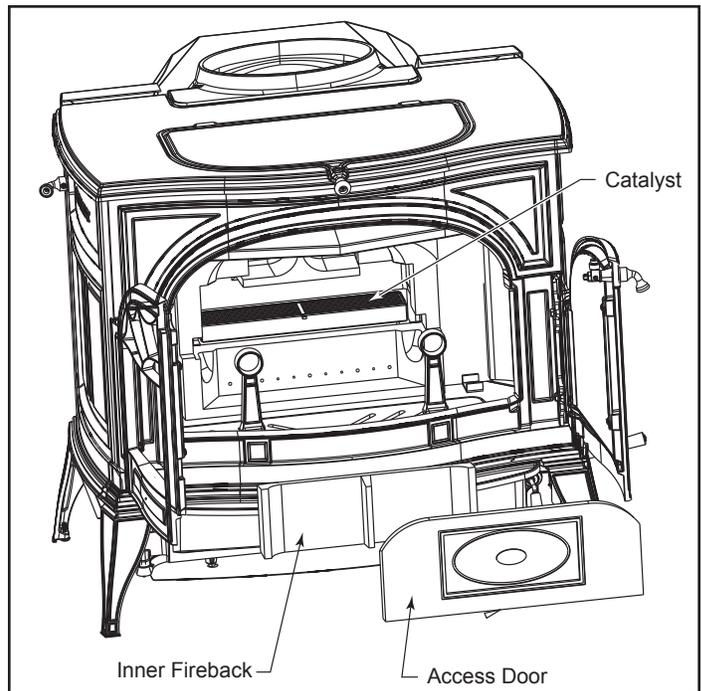
Figure 48 - Inspect the catalytic combustor.
