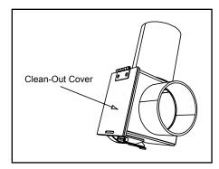
Figure 18.4 - Rear to Top Vent Adapter - 90°
