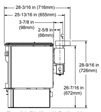
Figure 7.4 - Side View with Top Vent Adapter
