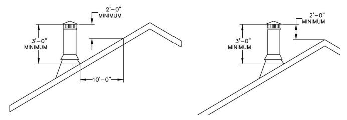
Figure 3 - Chimney Height Requirements
