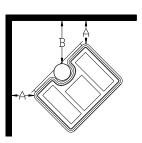
\* The National Fire Protection Agency has recommended minimum clearances to non-combustible surfaces. Following are two examples of NFPA 211 non-combustible walls. To make a wall non-combustible, protected it with a minimum of 24 gauge sheet metal or a minimum of 4" (102 mm) of masonry, both with a 1" (25mm) air space between the wall and the masonry or sheet metal. Refer
