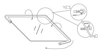
glass retainer clips. Remove the screws to separate the glass from the door.
