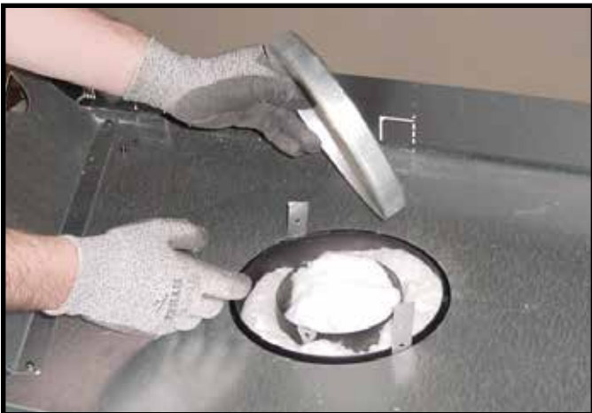
Figure 9.3 Remove the seal cap.
