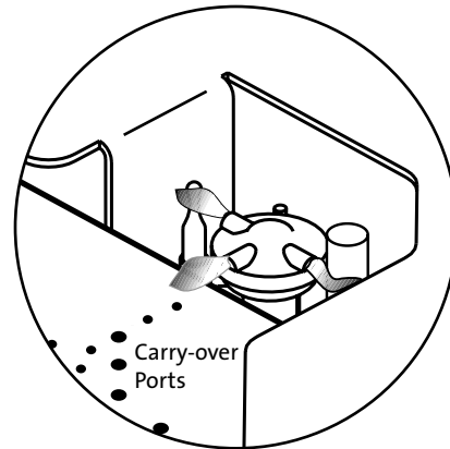
Figure 38a. Proper pilot flame appearance relative to burner carry-over porting.
