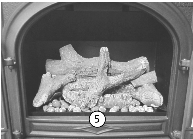
Figure 42. Place Ember Stones loosely over the burner plate. DO NOT OBSTRUCT THE GAS PORTING. SEE FIG. 43. Use the supplied rock wool sparingly.
