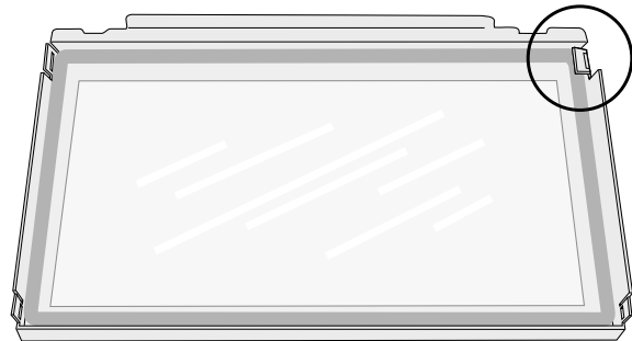
Figure 46. Bend the retainer tabs back enough to release the glass panel.
