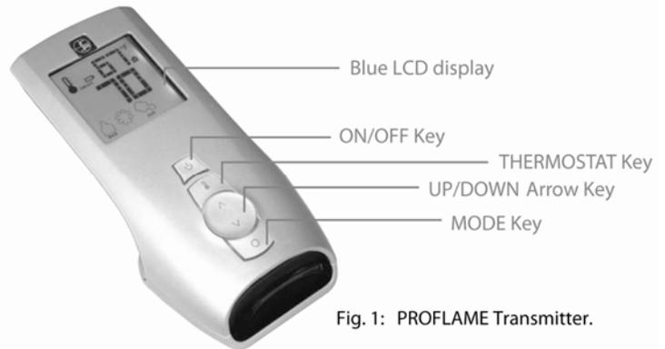
1. **ON/OFF KEY:** This button turns the system ON or OFF. When this button is pressed and the system is OFF, the pilot light will stay ON if the “Standing Pilot Switch” is in the ON position.
