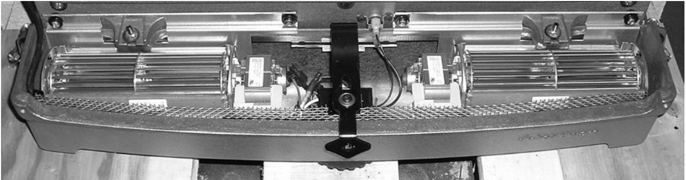
Photo 30 – Blower System (Ash Lip Cover Removed)
