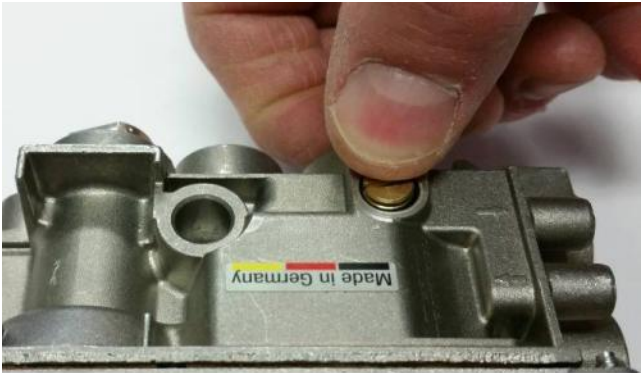
Figure 23 – NG Low Flow Screw Removal
