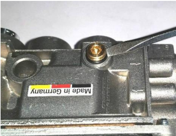
Figure 22 – Low Flow Orifice Removal – O-ring
