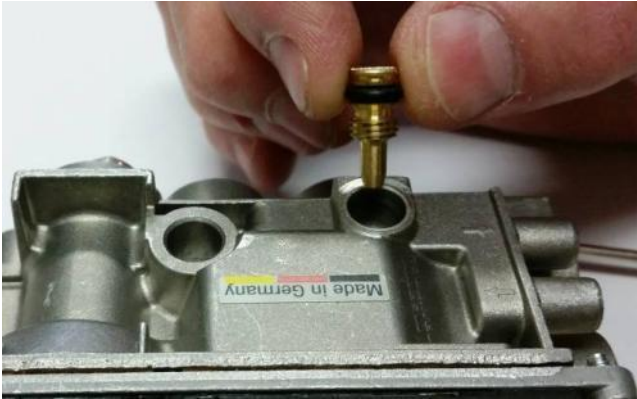
Figure 23 – NG Low Flow Screw Removal
