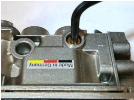
Figure 21 – Low Flow Orifice Removal
