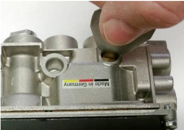
Figure 25 – Tighten LP Low Flow Orifice
